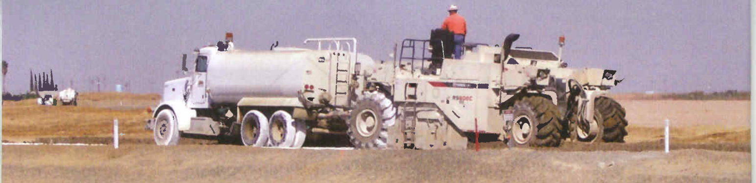
(Above) The excellent service from Herman equipment helps keep this sophisticated RS-600 productive. The Terex allows Griffin to hook up to the water truck with a 4" water hose. This allows for enough water for proper hydration.
